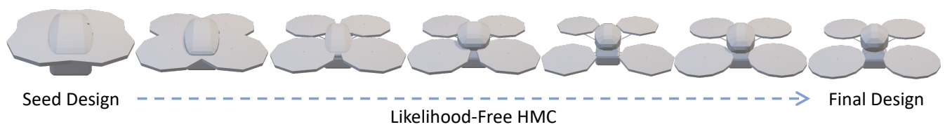
Figure 11: Sub-sampled quadcopter designs taken along the likelihood-free HMC chain using DNRE. The initial seed design on the far left has multiple structural interferences, including sensors that cut through the fuselage. As we move along the chain we see the design morph into our desired structure with very few interferences. This is achieved though increasing the arm length and changing the shape of the fuselage jointly with varying the placement of the interior sensing components.
